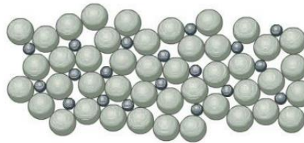
A model of the structure of steel
