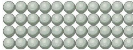
The diagram shows one way of modelling the atom arrangement in pure iron
