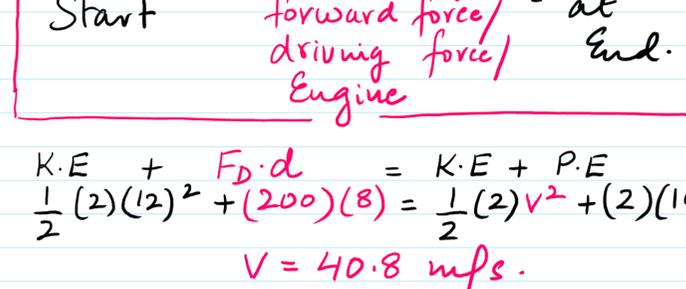
③ Energy at Start + W. done by forward force/ driving force/ Engine = Energy at End.
