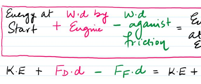
④ Energy at Start + W.d by Engine - W.d against friction = Energy at End
