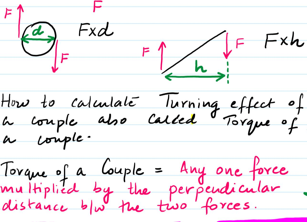
How to calculate Turning effect of a couple also called Torque of a couple.
