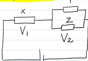
Suggest what happens to  $V_1$  &  $V_2$  if an extra resistor Z is added to the combination
