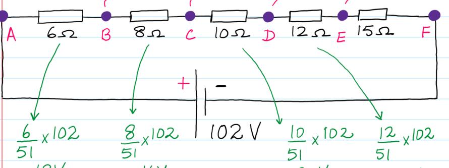
\* While moving from a higher potential (102V) towards a Lower potential (0V) calculate the voltage drop across each resistor using ratio theorem & keep on subtracting its voltage from the previous value.
