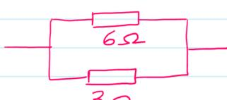
①  $\frac{1}{R_T} = \frac{1}{R_1} + \frac{1}{R_2}$  \* If only 2 resistors than total Resistance can also be obtained using
