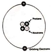
It is important to understand that the picture above is model of the atom. It conveys an impression of what the atom is like, but is not a completely true representation.
