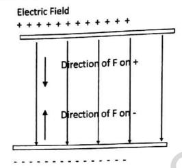
The direction of the force depends on the charge on the particle.
