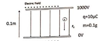
Find the velocity of the charge after it has travelled a distance of 5 cm. Use the following information:
