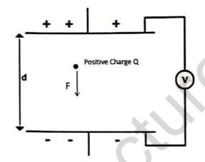
The field strength of the uniform field between charged parallel plates in terms of potential difference and separation.
