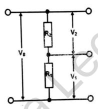
Figure: A potential Divider circuit
