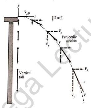
The speed in the x-direction is constant; in the y-direction the object moves with constant acceleration g.
