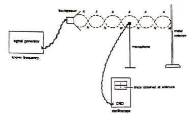
Stationary sound waves in air can be demonstrated using the set-up as shown above.
