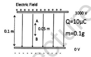
The work done by the field on the charge can be calculated easily because it is equal to the gain in kinetic energy by the charge.
