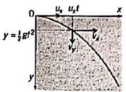
As an example, think about a particle sent off in a horizontal direction and subject to a vertical gravitational force (its weight). As
