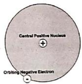
In this model the positive material is concentrated in a small but massive (lot of mass - not size) region called the nucleus. The negative particles (electrons) must be around the outside preventing the atom from trespassing on its neighbours space to complete this model. The diagram in next slide will help you to understand the results of the experiment.
