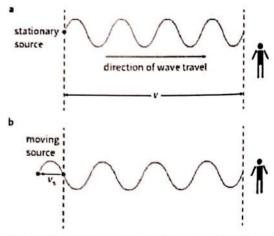
Figure 13.12 Sound waves, emitted at constant frequency by a a stationary source, and b a source moving with speedy, away from the observer.
