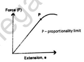
In the diagram above, if you extend the spring beyond point P, and then unload it completely; it won't return to its original shape. It has been permanently deformed. We call this point the elastic limit – the limit of elastic behavior.
