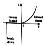
A diede is a device that has a low resistance in one direction (forward-biased direction) and a very high resistance in the other direction (reverse-biased direction). The I - V characteristic of a forward-biased semiconductor diede is similar to that of a thermistor, i.e. resistance decreases as p.d. increases
