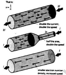
Figure 8.29 The mean drift velocity of electrons depends on the current, the cross-sectional area and the electron density of the material.
