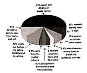
When carrying out practical work involving count – rates from radioactive sources, allowance should be made for this background radiation. This can usually be done effectively by measuring the background count in the laboratory for several minutes, and subtracting the appropriate amount from subsequent readings taken with the source.
