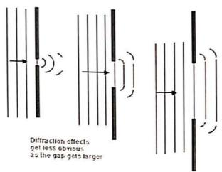
It is the relative sizes of the aperture to the wavelength that is important.
