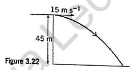
To find the time t for which the stone is in the air, work with the vertical component of the motion, for which we know that the initial component of the motion, for which we know that the initial component of velocity zero, the displacement y = 45 m, and the acceleration a is 9.81 ms<sup>-2</sup>. The
