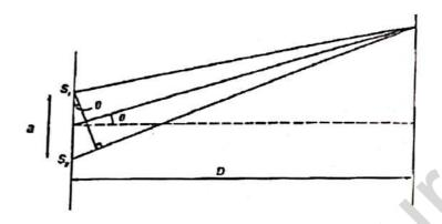
In the double slit experiment; bright & dark fringes alternate at equal separation.
