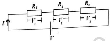
Figure Resistors in series-Note the current through ah the resistors is the same but voltage is not When a potential difference V is applied across the series the current through all the resistors is the same, but the potential difference across each resistor is different and the sum of these individual
