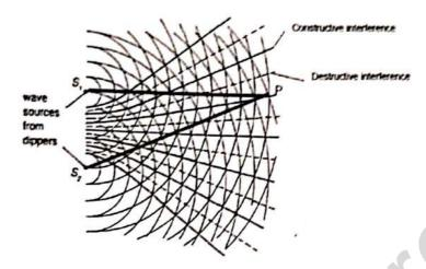
The 2 thick lines intersecting at P represent the paths of water waves from the 2 sources to produce a constructive interference at P.
