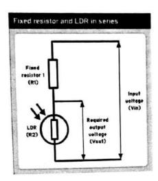
Figure 10: LDR used in a potential divider
