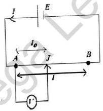
Figure 11: A variable voltage potential divider the potential drop increases.hence by varying the length of AJ the potential can be varied. Let be the resistivity of the wire AB and let E be 5mf of the battery,let Io be the length of wire AB and let I be the length AJ then
