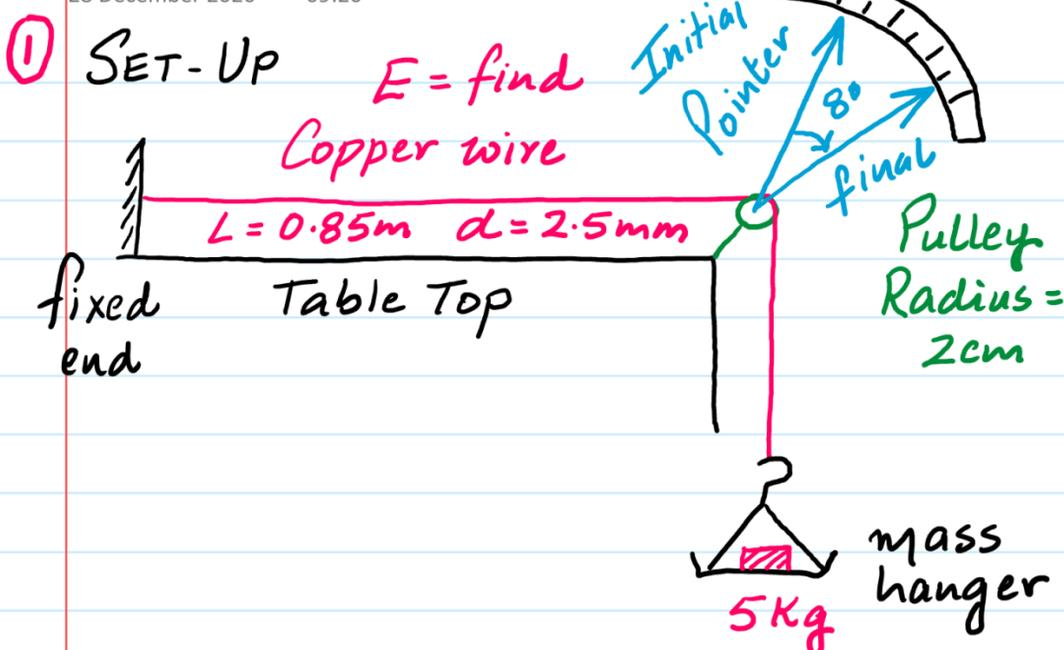
As mass is placed in the mass hanger, the pointer deflects (due to extension of the wire) by  $8^\circ$  as shown above
