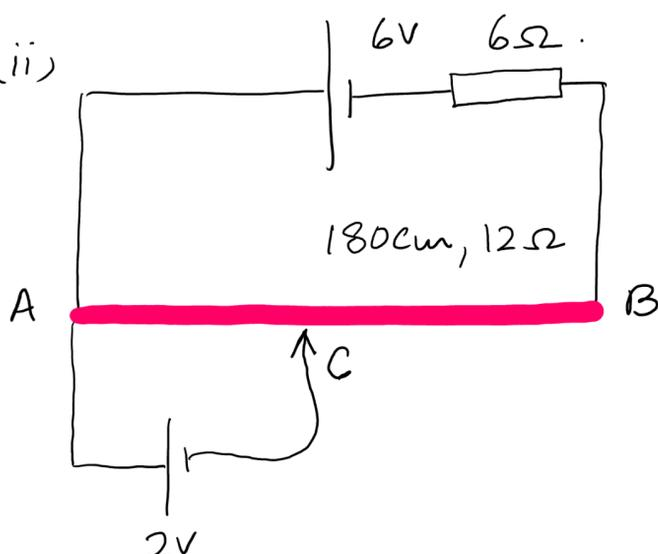
Cal. the new length of AC now required if an additional 6Ω resistor is placed with the Primary cell.
