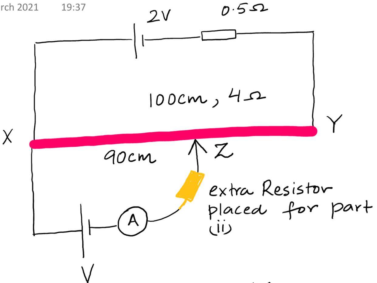
(i) If that (A) reads 0A (null deflection). Calculate the unknown voltage V?
