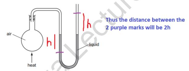
The flask is now gently heated and the liquid level in the right-hand side of the U-tube rises through a distance h. The density of the liquid is  $\rho$ .
