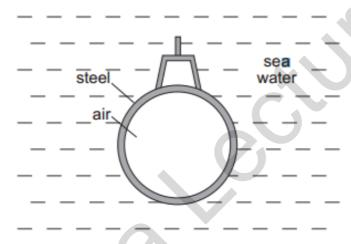
What causes the upthrust on the submarine?
