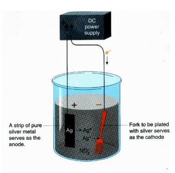
The coating of a metal object with another metal object is called Electroplating. It is carried out in a cell called plating bath. It contains an electrolyte. For silver plating electrolyte is a solution of silver salt. The article to be plated is made the cathode in the cell so that metal ions move to it when current is switched on.
