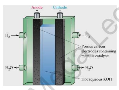
A fuel cell consists of two electrodes consisting of a negative electrode (or anode) and a positive electrode (or cathode) which are sandwiched around an electrolyte (conducting
