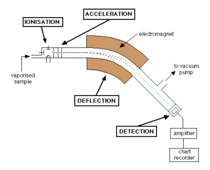
Knowledge of the working of the mass spectrometer is **not** required by CIE.
