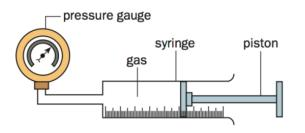
The pressure of the gas inside the syringe is increased by slowly pushing the piston inwards (to compress the gas).
