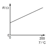
The resistance of the wire at 0  $^{\circ}$ C is 1.00  $\Omega$  and at 100  $^{\circ}$ C is 1.40  $\Omega$ .
