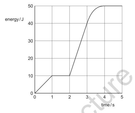
What is the maximum electrical power generated at any instant during these first 5 seconds?
