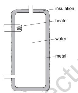
Water at the bottom of the tank stays cold for some time.
