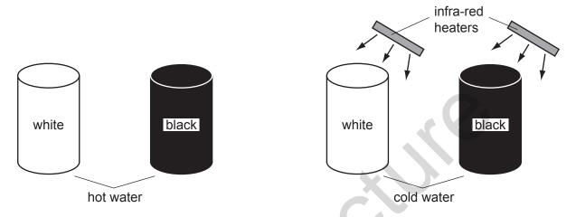
The hot water in the black can cools more quickly than the hot water in the white can. The cold water in the black can heats up more quickly than the cold water in the white can.
