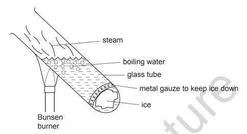
Why does the ice take a long time to melt, even though the water at the top of the tube is boiling?
