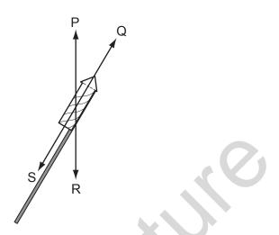
As the rocket flies through the air, three forces act on it. These forces are weight, thrust and air resistance.
