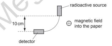
Which particles are deviated and reach the detector?
