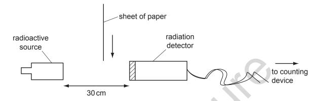
The experimenter moves the paper between the source and the detector. There is no difference in the count-rate.
