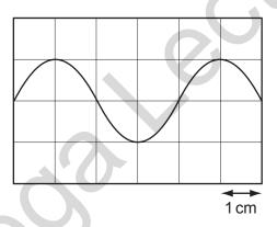
What is the time for one complete rotation of the coil of the generator?
