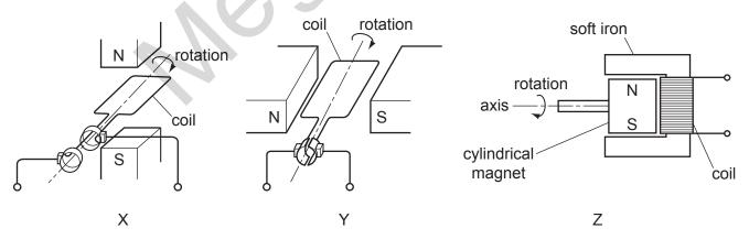
Which devices provide an alternating current (a.c.) output?
