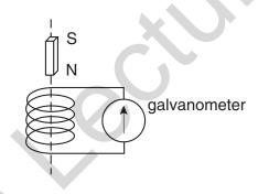
The magnet moves through the coil and, as it falls away from the coil, the galvanometer pointer
