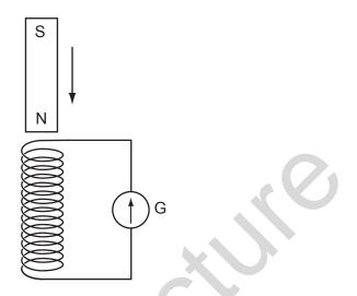
When a magnet is allowed to fall towards the coil, the galvanometer pointer gives a momentary deflection to the right of the zero position.
