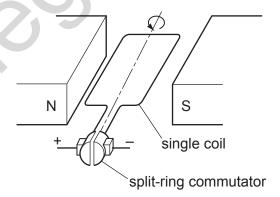
The split-ring commutator reverses the current in the coil as the coil rotates.
