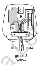
What is the effect of using the plug wired in this way?
