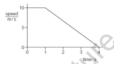
Vhat is the distance travelled by the car in the four seconds?
