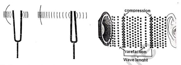
2. The sound travels in the form of longitudinal waves. The wave consists of a series of compressions, C followed alternately by rarefactions, R.
