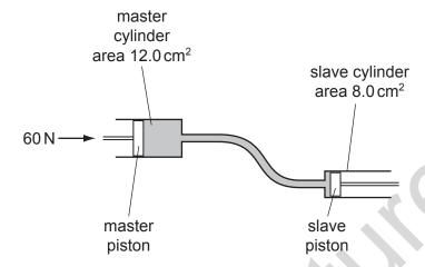
The cross-sectional area of the master cylinder is  $12.0 \, \text{cm}^2$  and the cross-sectional area of the slave cylinder is  $8.0 \, \text{cm}^2$ . The force applied to the master piston is  $60 \, \text{N}$ , producing a pressure of  $5.0 \, \text{N/cm}^2$ .
