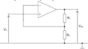
As before, the current in the two resistors are equal and can be written as
