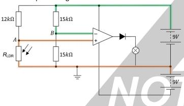
• In daylight, LDR has low resistance (3k $\Omega$ ) & noninverting voltage is small causing op-amp to be negatively saturated (-9V). Diode reverse-biased: <u>lamp</u> doesn't light
