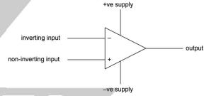
The output is proportional to the difference between the two input voltages, given by:
