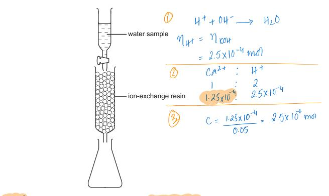
A 50 cm<sup>3</sup> sample of water containing dissolved calcium sulphate was passed through the ionexchange resin. Each calcium ion in the sample was exchanged for two hydrogen ions. The resulting acidic solution collected in the flask required 25 cm<sup>3</sup> of  $1.0 \times 10^{-2}$  mol dm<sup>-3</sup> potassium hydroxide for complete neutralisation.
