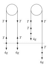
Both this and the falling ball problem illustrate how the 'work-energy' or 'conservation of energy' methods can be used to solve the problem, rather than using Newton's Second Law of motion . This is because, in these examples, you are interested in the speed as a function of distance, and energy methods are quicker in this situation.
