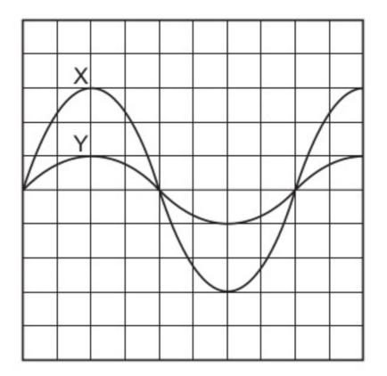
Signal X has a frequency of 50 Hz and peak voltage of 12 V.
