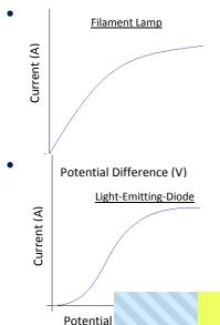
This is known as non ohmic; the current is not proportional to the potential difference. This is because the temperature changes as increased current passes through the filament. It is ohmic for small potential differences This is also non ohmic. For values of up to about 2 volts (depending on the colour of the L.E.D) the current remains at 0, so the resistance can be said to be infinite. Above 2 volts, the resistance decreases to
