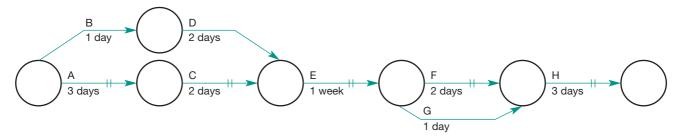
Figure 27.2 Adding durations to find the critical path
