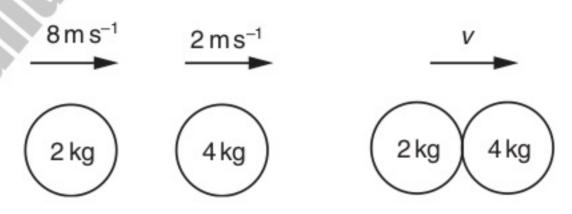
After collision, both balls move at the same velocity v.
