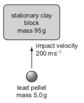
The pellet hits the block with an initial velocity of 200 m s<sup>-1</sup>. It embeds itself in the block and does not emerge.
