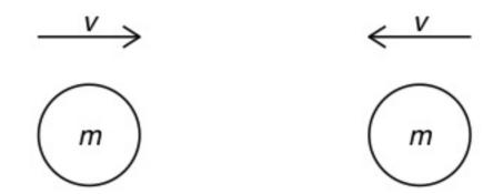
The spheres have a head-on elastic collision.
