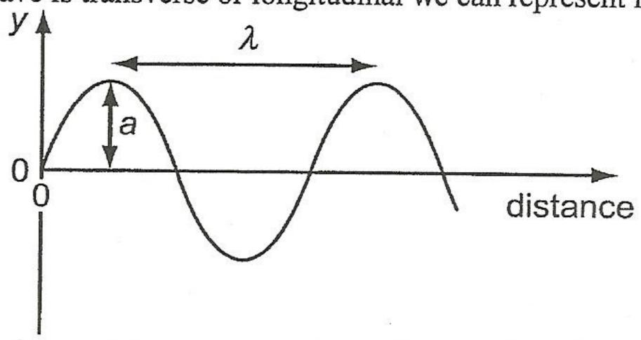
The displacement of a particle on a wave is its distance from its rest position, and the amplitude of a wave is its maximum displacement from its rest position.
