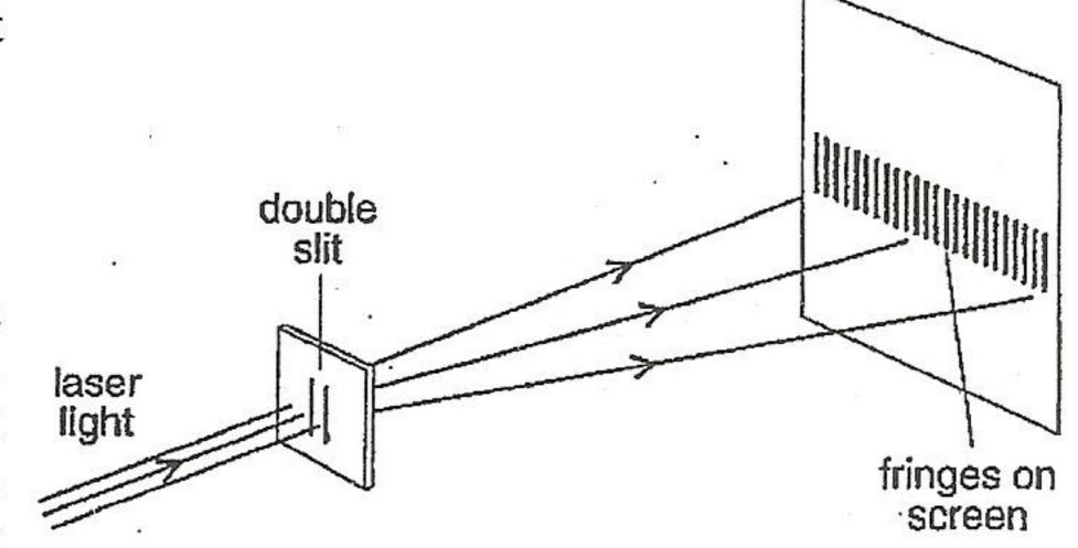
experiment. The maximum intensity of the double slit double slit remains the same, the fringe width is narrower hence it is sharper and the double slit pattern fades away at every single slit.
