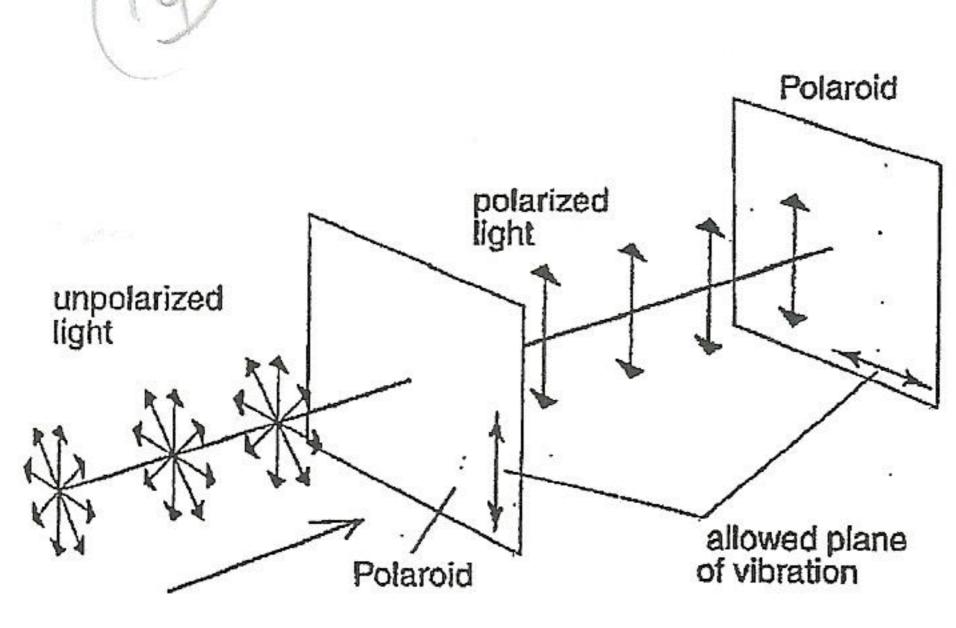
Unpolarized light may be polarized by passing it through a thin plane. Hence for a plane to be polarized is for the vibration to be contained in one plane only.
