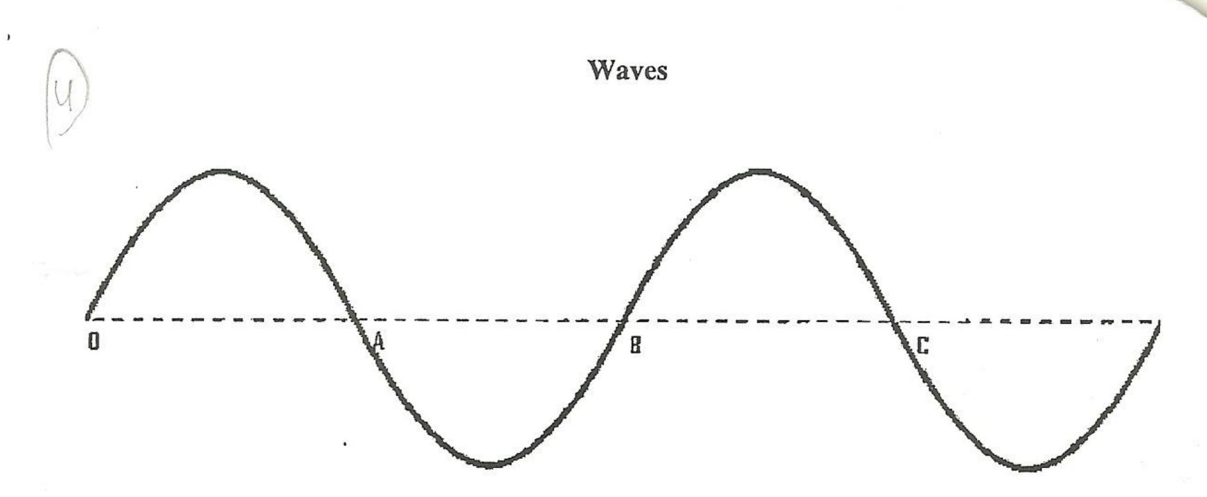
'A' vibrates 'T' seconds after 'O' because distance between them is  $\lambda$  and time is T. When a wave passes, the particles along the path of the wave starts to vibrate with time, there is lagging behind in the vibrations. For e.g. the particle B will start to vibrate T seconds later than O and they are separated by a distance  $\lambda$ . O & B are said to have a phase difference.
