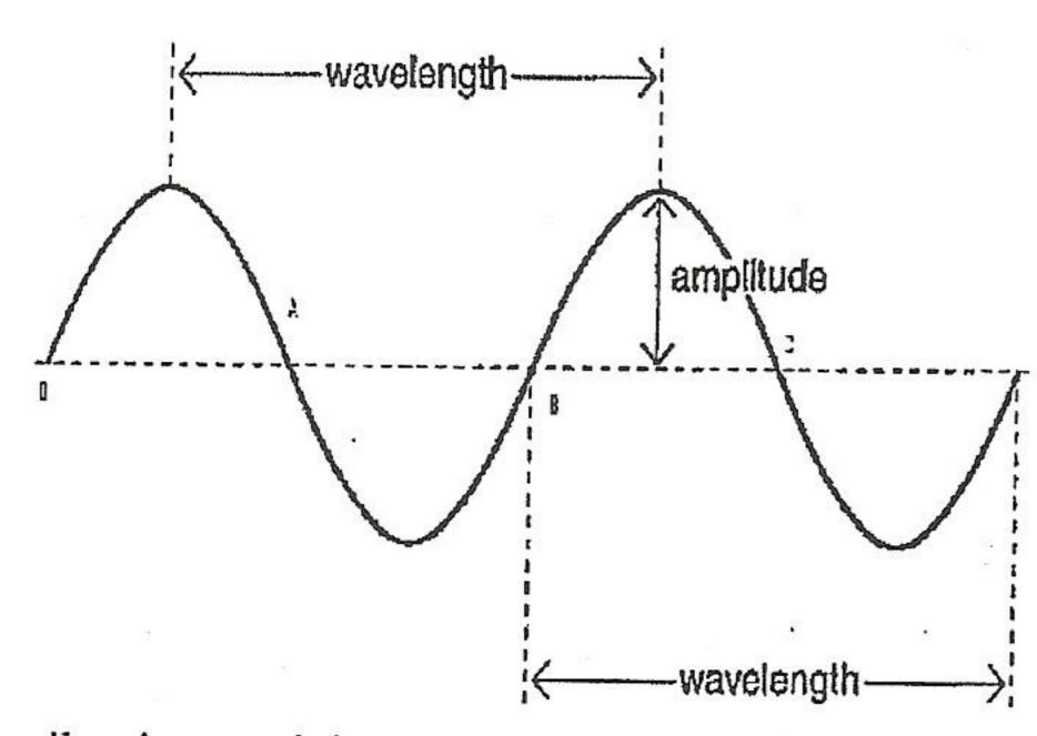
This graph shows how different particles along the path of the wave are displaced at a given instance.
