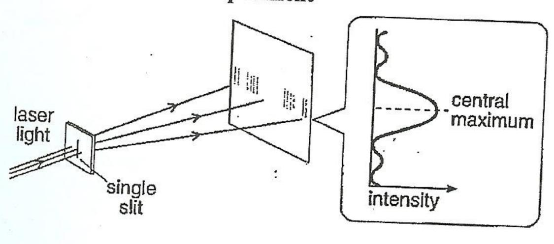
When a point of source of light is viewed through a narrow slit alternate bright
