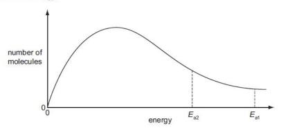
$E_{\rm a}$  is the activation energy for the reaction between the gases. Of the two values shown, one is for a catalysed reaction, the other for an uncatalysed one.
