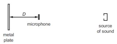
Sound of the unknown frequency is reflected back from a metal plate. A microphone placed at a distance D from the metal plate detects the sound intensity. A minimum intensity is detected with  $D = 12.0 \, \text{cm}$ . The plate is moved further away from the microphone until the next minimum is detected with  $D = 15.0 \, \text{cm}$ .
