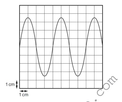
The oscilloscope time-base setting is 0.5 ms cm<sup>-1</sup> and the Y-plate sensitivity is 2 V cm<sup>-1</sup>.
