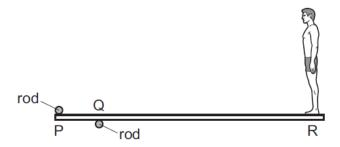
The forces exerted by the rods on the board are vertical. The board remains in equilibrium as the person slowly moves towards point Q from end R.
