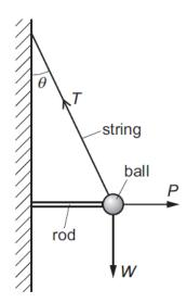
The string is at an angle  $\theta$  to the vertical. The tension in the string is T. The ball is held away from the wall by a horizontal force P from a metal rod.
