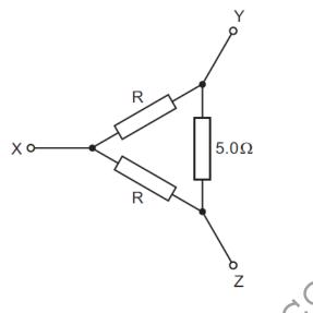
The resistance between Y and Z is found to be  $2.5 \Omega$ .
