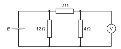
The voltmeter has a very high resistance and reads a potential difference  $V_{\mathrm{out}}$ .
