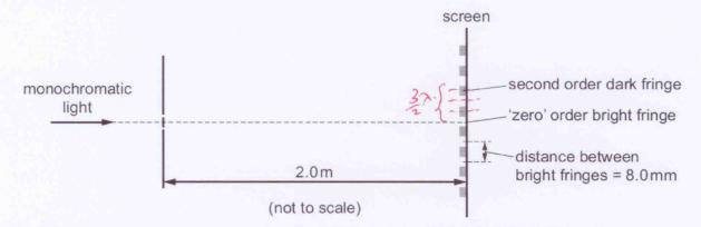
What is the path difference between the light waves from the two slits that meet at the second order dark fringe?
