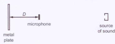
Sound of the unknown frequency is reflected back from a metal plate. A microphone placed at a distance D from the metal plate detects the sound intensity. A minimum intensity is detected with D = 12.0 cm. The plate is moved further away from the microphone until the next minimum is detected with  $D = 15.0 \,\mathrm{cm}$ .
