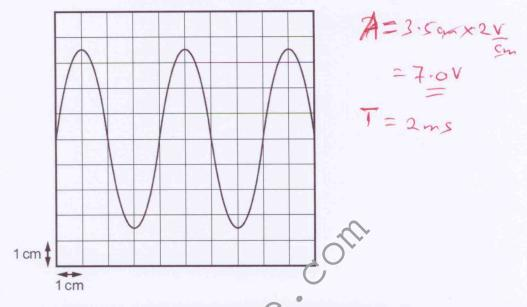
The oscilloscope time-base setting is  $0.5\,\mathrm{ms\,cm^{-1}}$  and the Y-plate/sensitivity is  $2\,\mathrm{V\,cm^{-1}}$ .
