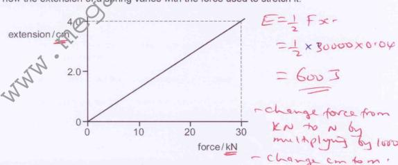
What is the strain energy in the spring when the extension is 4.0 cm?
