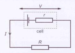
When the internal resistance r of the cell increases, what is the effect on V and on I?
