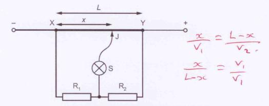
J is moved along XY to a point at which the lamp is off. This point is at a distance x from X.
