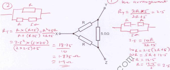
The resistance between Y and Z is found to be  $2.5 \Omega$ .
