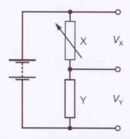
The potential difference across resistor X is  $V_X$  and the potential difference of resistor Y is  $V_Y$ .
